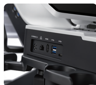
Top-access I/O ports enable visual alignment and insertion
